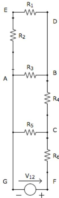
$$R_1 = R_2 = R_3 = R_4 = R_5 = R_6 \\ = R = 120 \Omega$$
