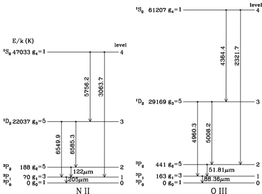
**Figure 4.1** Energy-level diagram for the ground configuration of the  $2p^2$  ions N II and O III. (Fine-structure splitting is exaggerated for clarity.) Forbidden transitions connecting these levels are shown, with wavelengths in vacuo.
