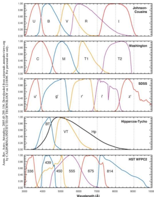
Figure 1 Schematic passbands of broad-band systems.
