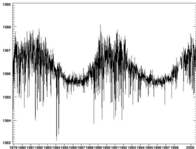
**Figure 1.6.** Plot of the Solar Constant (in  $\text{W m}^{-2}$ ) as a function of time from satellite data. The variation follows the 11-year Sunspot cycle such that when there are more sunspots, the Sun, on average, is brighter. The peak to peak variation is less than 0.1 per cent. This plot provides definitive evidence that our Sun is a variable star. (Reproduced by permission of [www.answers.com/topic/solar-variation](http://www.answers.com/topic/solar-variation))
