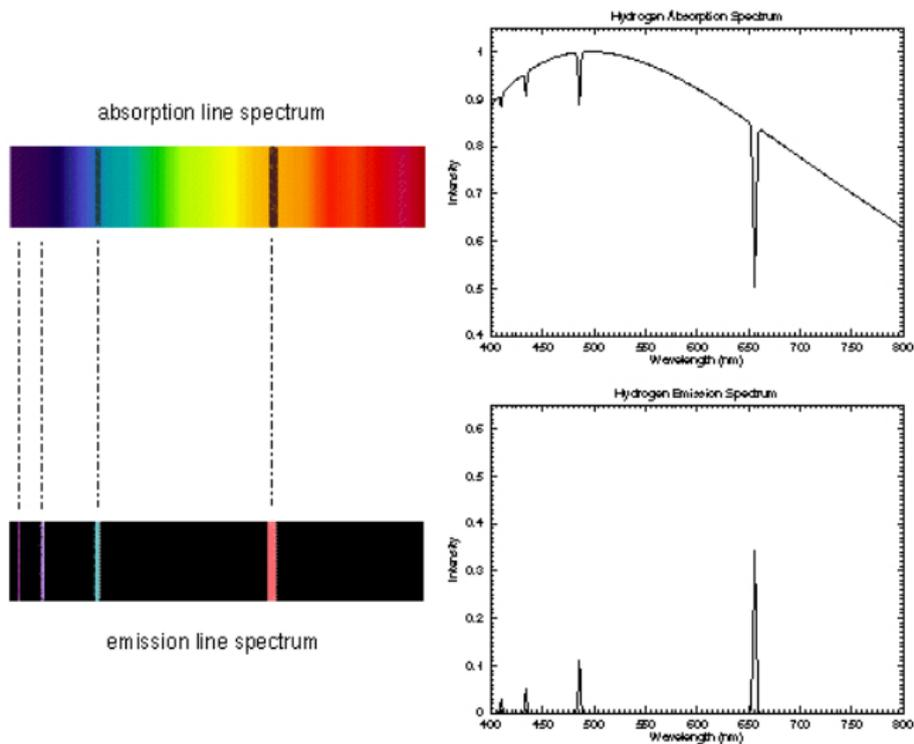
Two ways of showing the same spectra: on the **left** are pictures of the dispersed light and on the **right** are plots of the intensity vs. wavelength. Notice that the pattern of spectral lines in the absorption and emission line spectra are the **same** since the gas is the same.
