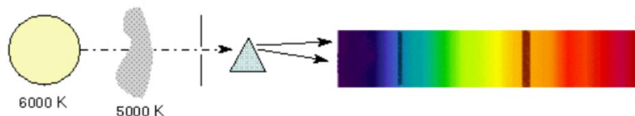
Type of spectrum seen depends on the temperature of the thin gas **relative to** the background. TOP: thin gas is *cooler* so **absorption lines** are seen.
