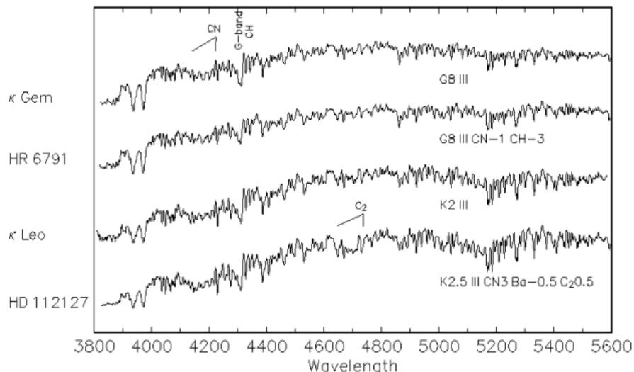
**FIGURE:** HR 6791 = G8 III ( $\kappa$  Gem = G8 III standard) with weak CN 4216 Å band, and very weak G-band (CH). HD 112127 = K2.5 III ( $\kappa$  Leo = K2 III standard), has an exceptionally strong CN 4216 Å band, and shows the 4737 Å C<sub>2</sub> Swan band, and a clear depression of the continuum in the vicinity of 5200 Å, most probably due to the 5165 Å C<sub>2</sub> Swan band.
