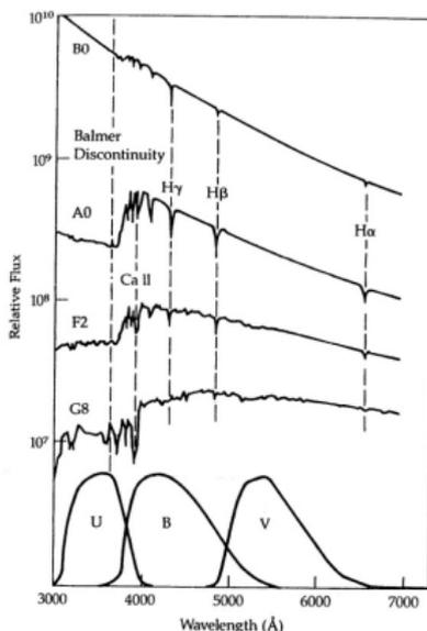
**FIGURE** Profiles of the spectra of various classes of main-sequence stars compared to the *UBV* bandpasses. Note that the Balmer discontinuity falls in the *U* but not the other filters. This nonlinear effect causes the sharp bend in color-color plots.
