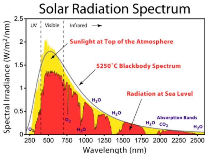
Figure 1 Electromagnetic spectrum of sunlight above and below the atmosphere.
