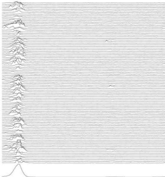
100 single pulses from the 253-ms pulsar PSR B0950+08 and pulse profile averaged over 5 minutes ( $\sim 1200$  pulses)
