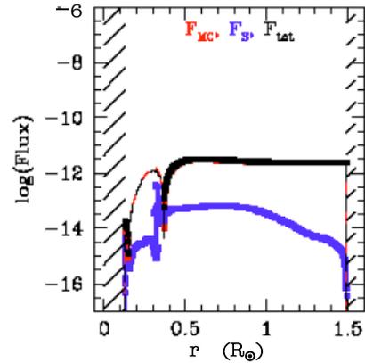
Figure 5. Logarithm of the total flux of angular momentum (black line) and of that transported by meridional circulation,  $F_{MC}(r) = \frac{1}{R_\odot^4} \frac{1}{5} \rho r^4 \bar{\Omega} U_2$ , (red line) and by shear-induced turbulence,  $F_S(r) = \frac{1}{R_\odot^4} \rho \nu_v r^4 \partial_r \bar{\Omega}$ , (blue line).
